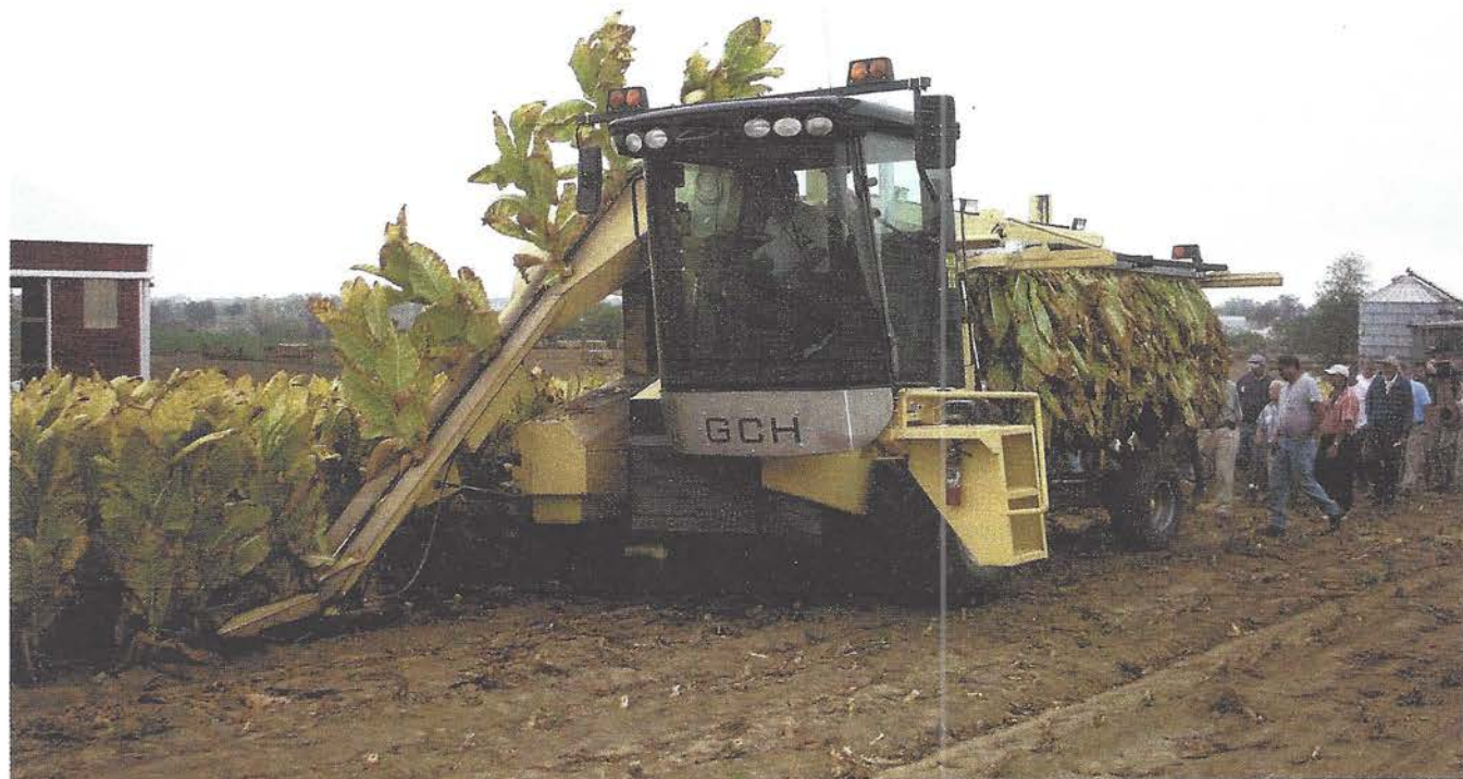
GCH's automatic burley harvester helps farmers reduce labor requirements by up to 80 percent.
