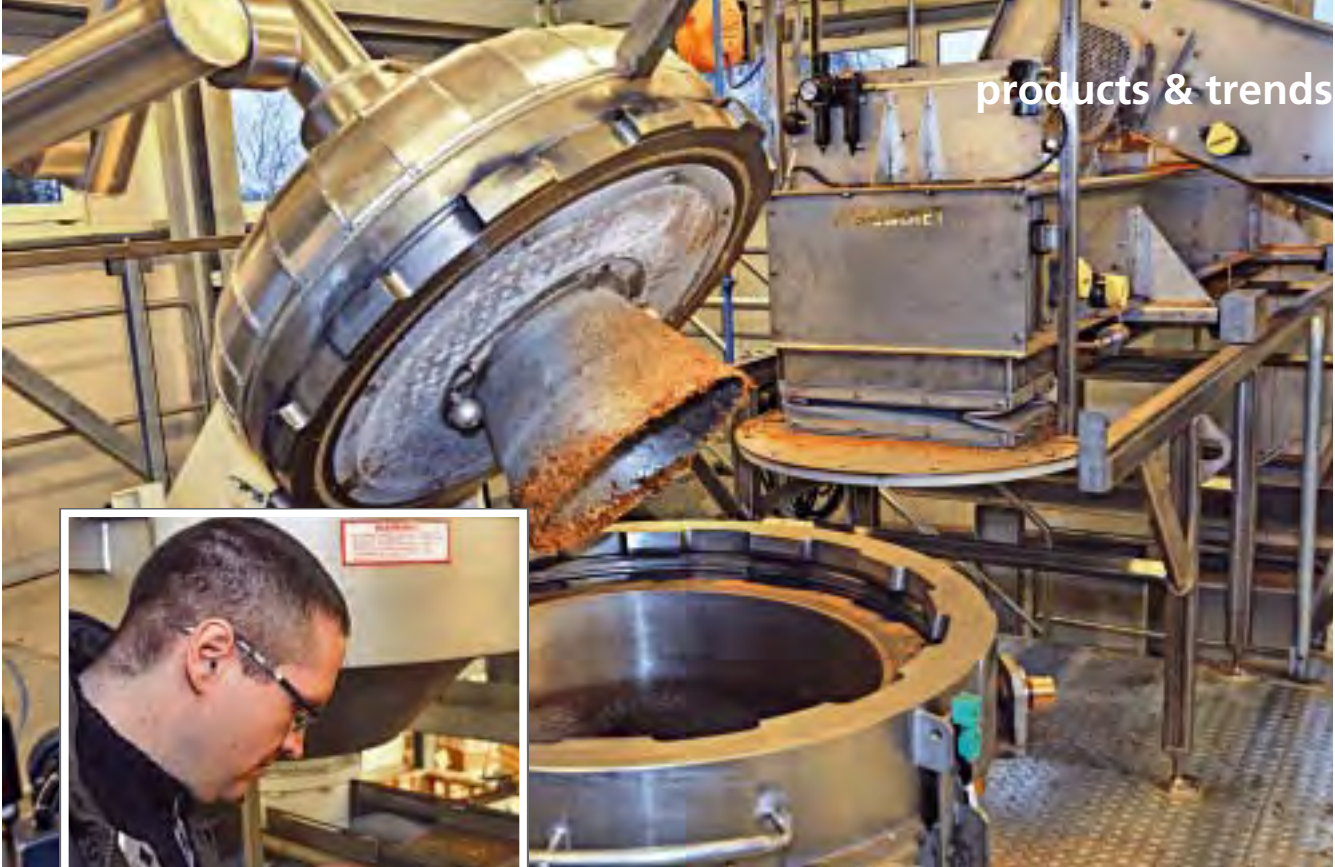
The DIET impregnator lid closes on a load. Peter Steinhauser, electrical and primary maintenance manager, demonstrates how cold DIET expands in response to the warmth from his hand.
